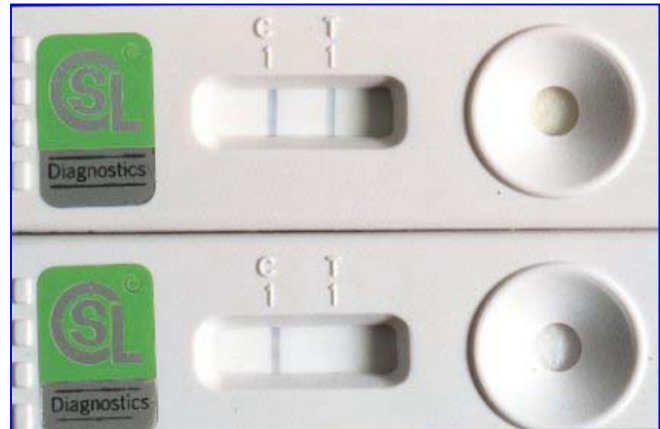
Figure 3: Development of the LFD test result (Danks and Barker, 2000). An actual positive and negative result using a Pocket Diagnostic device (results obtained after 3 minutes after sample addition) +ve (2 blue lines - control and test (C and T)) indicates a positive result; -ve (1 blue line - control only (C)) indicates a negative result
