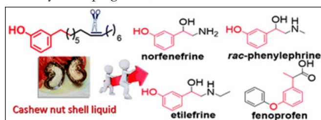
Figure 3: Synthesis of pharmaceutical drugs from cardanol derived from CNSL
