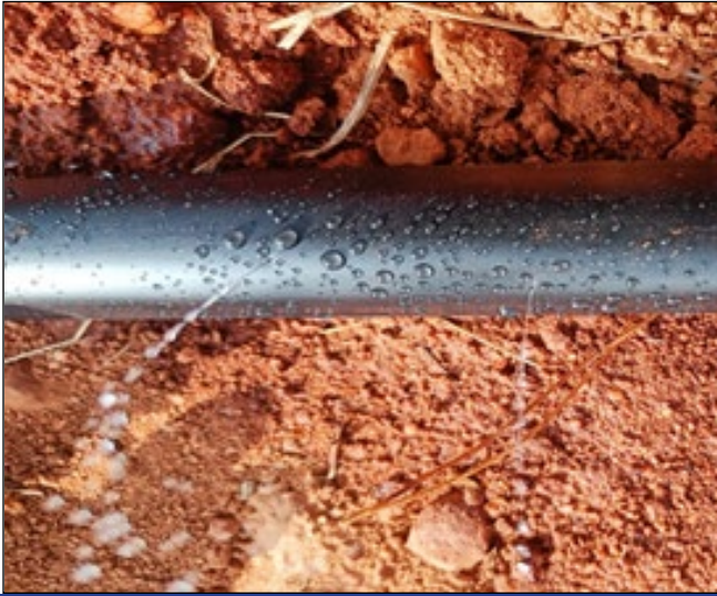
Figure 7: Rain pipe with punched laser holes
