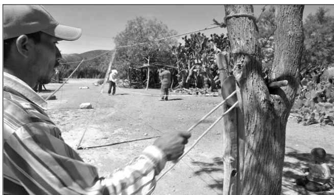
Twisting of the grown rope by using a local man made wooden pulley held between two poles
