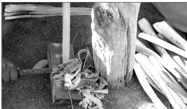
Use of an unsharpened knife, a flat piece of wood known as “banco” and a wooden pole which holds the tip of the knife during the shredding process.
