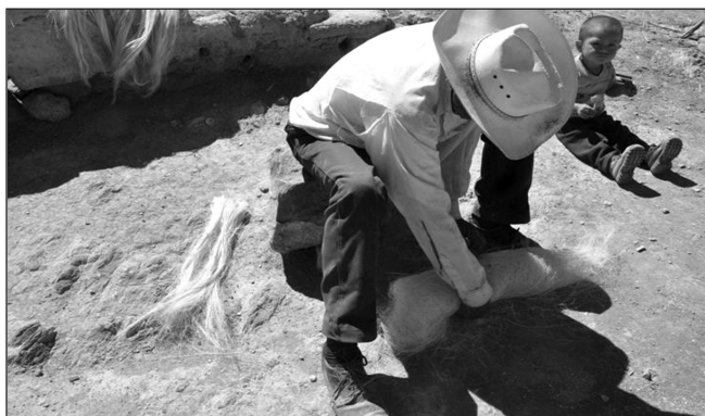
Rolling unraveled Agave lecheguilla fiber to begin the thread of a rope
