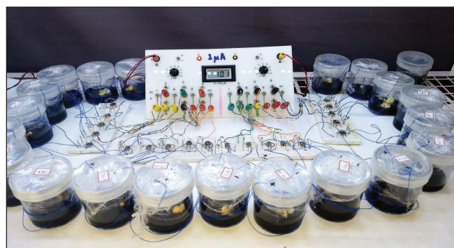
Figure 5: Experiment setup – 1 \mu\text{A} for 20 channels
