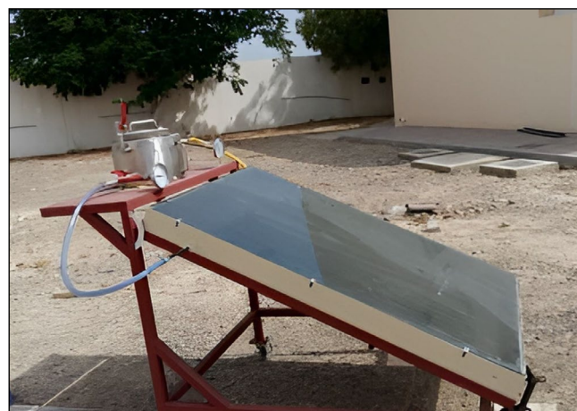
Figure 3: Solar pasteurization system with the aid of flat-plate collector (Saad et al., 2021)
