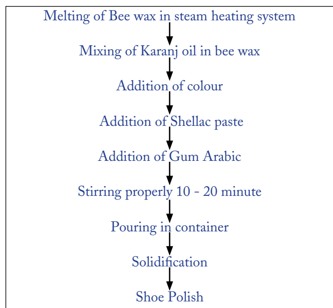
Figure 1: Flow chart of making shoe polish
