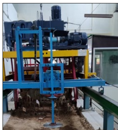
(a) Test trolley, processing trolley and vertical rotor
