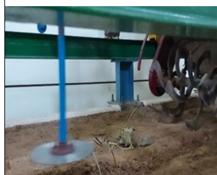
(d) Simulated samples in stem holder during cutting
