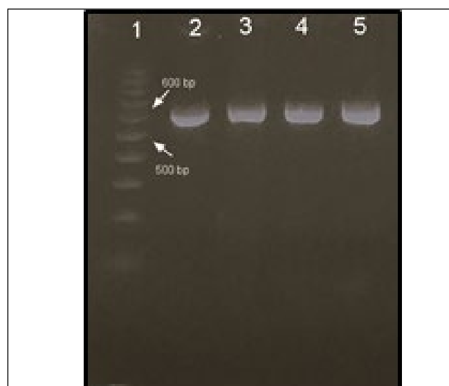
Plate 1: Results of PCR showing 16 S rRNA gene of E. coli Lane 1: 100 bp ladder; Lane 2: Positive control; Lane 3-5: Positive samples (Size 585 bp)
