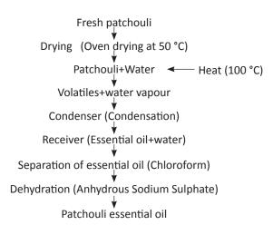
Figure 1: Flow diagram of patchouli oil extraction process
